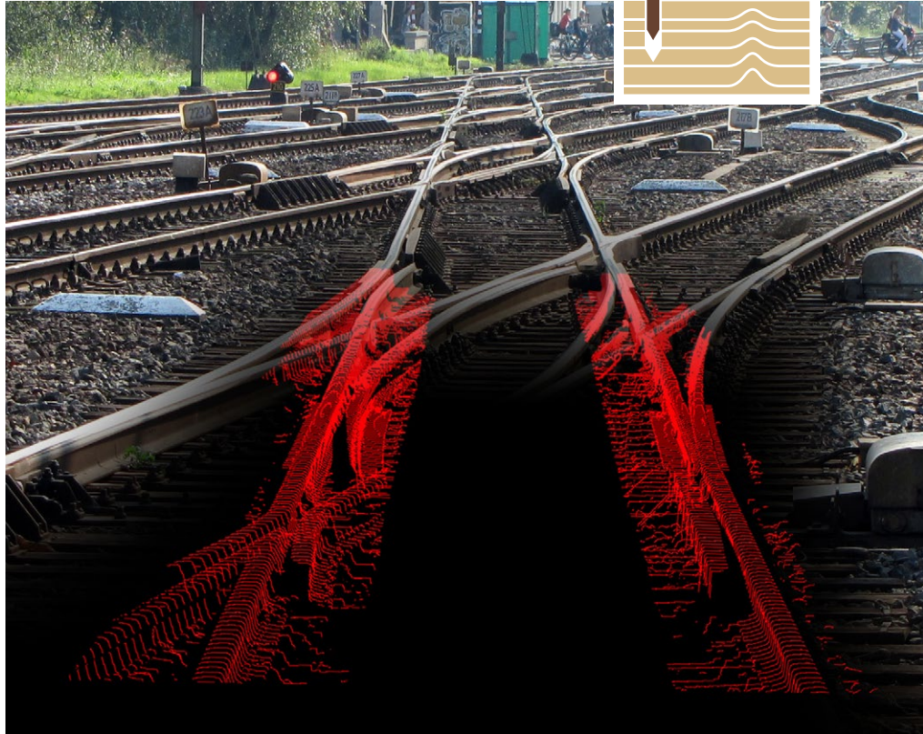
Fugro's RILA system gathers absolute and relative position, rail wear and video information.
